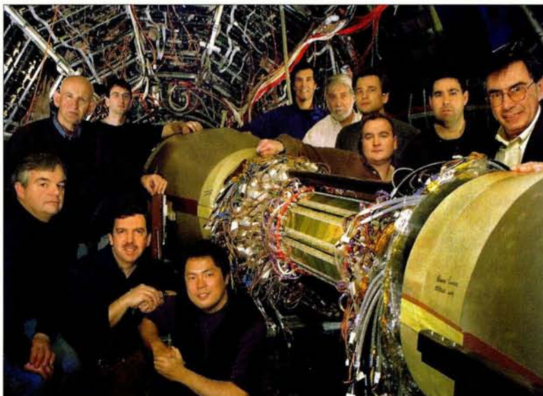
The STAR Silicon Vertex Tracker prior to insertion in the STAR Time Projection Chamber. Also shown is the team that was leading the construction and the installation of the detector. From left to right are Rolf Beuttenmuller (Brookhaven), Veljko Radeka (Brookhaven), Robert Willson (Ohio State), Phil Kuczewski (Brookhaven), Jun Takahashi (São Paulo), Robert Soja (Brookhaven), Bill Leonhardt (Brookhaven), Rene Bellwied (project leader, Wayne State) and David Lynn, Don Pinelli, and Tom Ludlam (Brookhaven).
