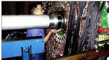
H1's new proportional chamber being inserted into the central detector assembly.
