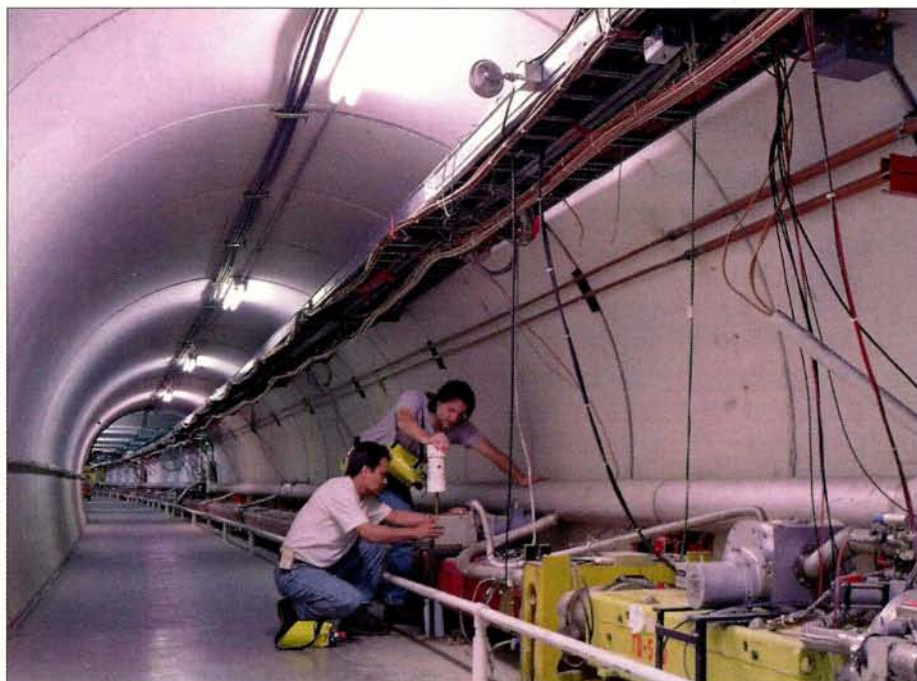
Part of the 4-mile tunnel housing Fermilab's superconducting Tevatron proton-antiproton collider, which is now running for physics at 980 GeV per beam (1960 GeV collision energy). The tunnel was originally built for Fermilab's Main Ring, which has now been removed.
