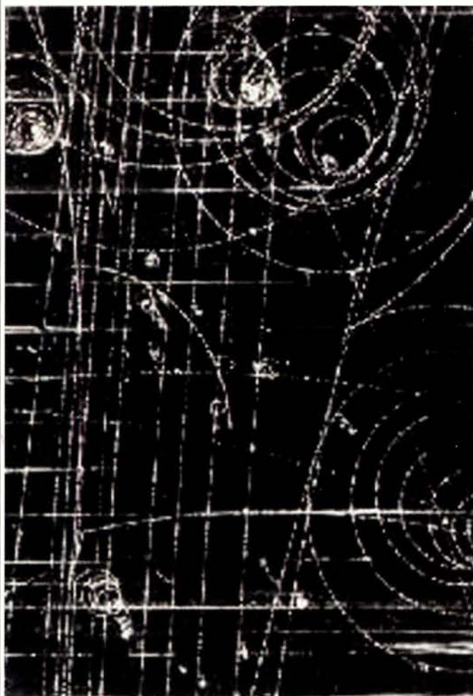
Fig. 6. 1964 – the bubble chamber classic, the production and decay of the \Omega^- hyperon in Brookhaven's 2 m bubble chamber. This remarkable event permitted reconstruction of all particle momenta and the determination of the mass of the \Omega^- .
